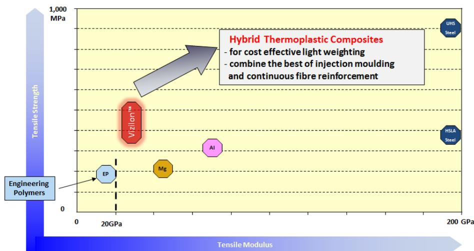
Figure 10: Mechanical property advantage of Vizilon® over traditional materials [3]
