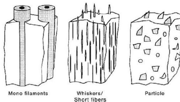
Figure 6-2: Schematic presentation of three shapes of metal matrix composite materials [2]
