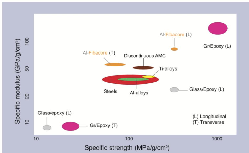
Figure 8: Strength advantages of AL Fibacore [4]
