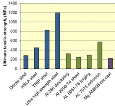
Figure 1: Mechanical properties for commonly used casing materials.
