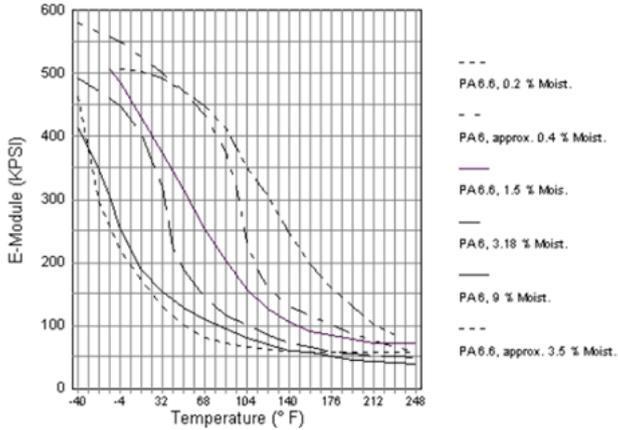
Figure 4: Effect of Temperature & Moisture Content on E-Modulus of PA 6 & 6.6 (www.intechpower.com)
