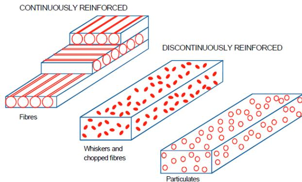
Figure 2-2: Composite reinforcement Types [1]
