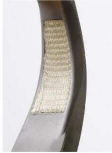
Figure 9: Al Fibacore insert positioned on an aluminium casing. [4]
