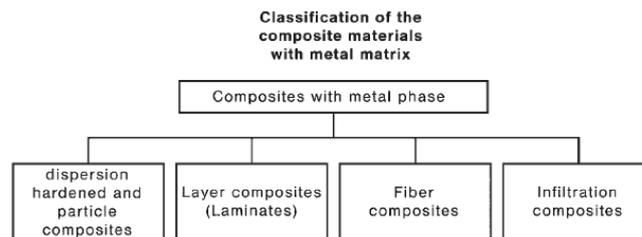
Figure 6-1: Classification of composite materials with metal matrixes [2]
