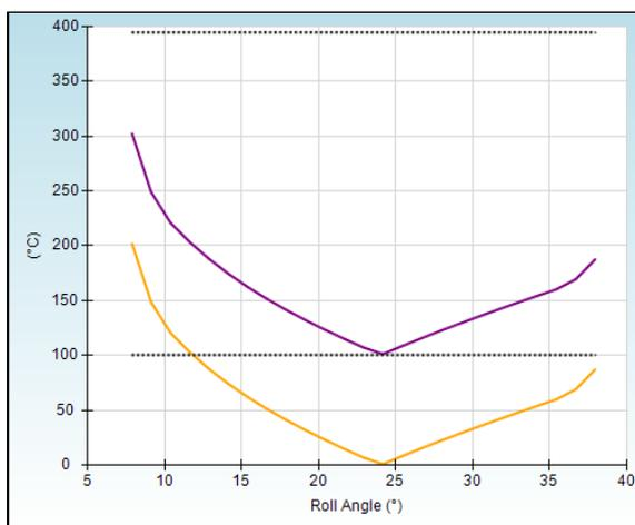
Figure 3 – Lubricant Flash Temperature without Micro-Geometry
