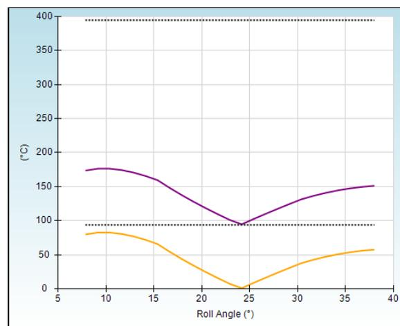
Figure 4 – Lubricant Flash Temperature with Micro Geometry
