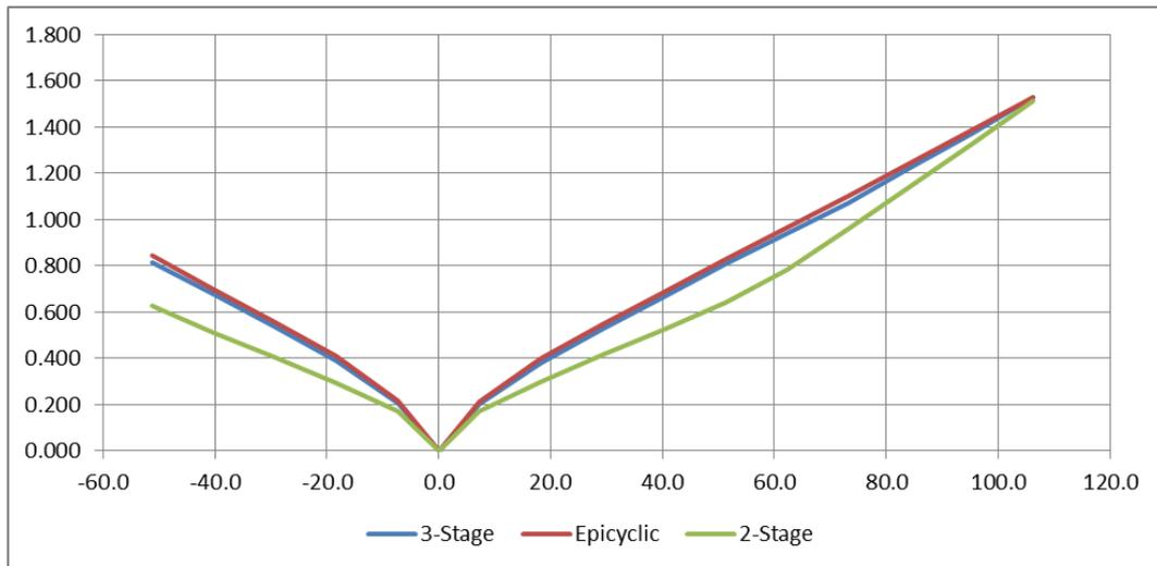
Figure 2 – Transmission Power Loss at 7000 rpm Input Speed
