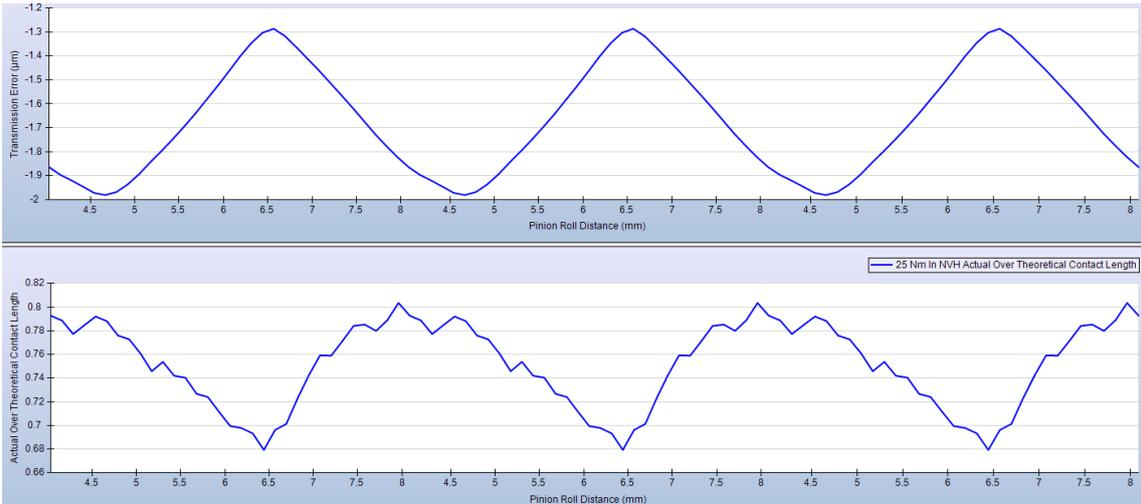
Figure 5 – Transmission Error and Tooth Contact Length Variation
