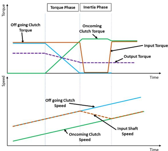
Figure 1: Power On Upshift diagram
