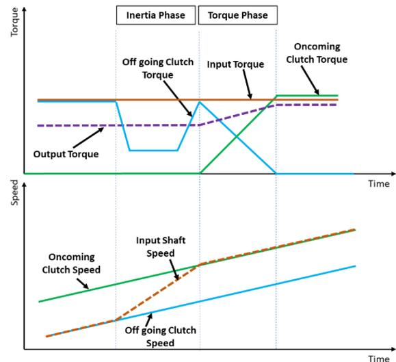
Figure 2: Power On Downshift diagram
