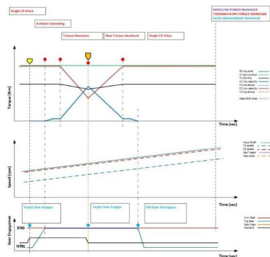
Figure 6: Change of mind shift implementation in Infinite Control during torque phase
