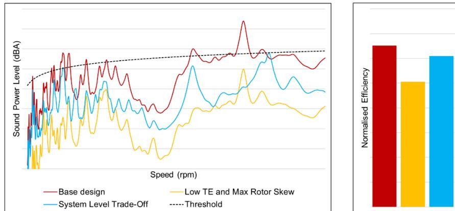
**Fig. 6.** Sound power level analysis of a powertrain optimised for NVH at a system-level
