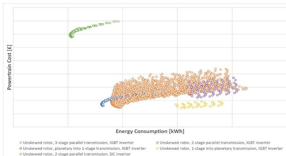
**Fig. 2.** ePOP results depending on the choice of power inverter and transmission
