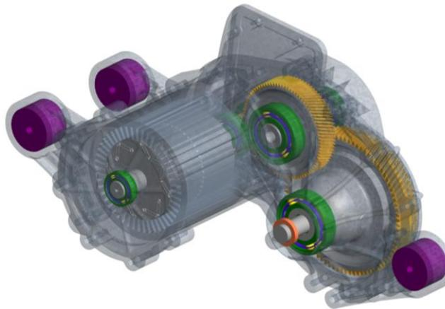
**Fig. 4.** 3D MASTA model of the designed powertrain
