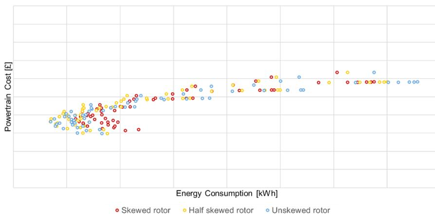
**Fig. 3.** ePOP results depending on the choice of rotor design
