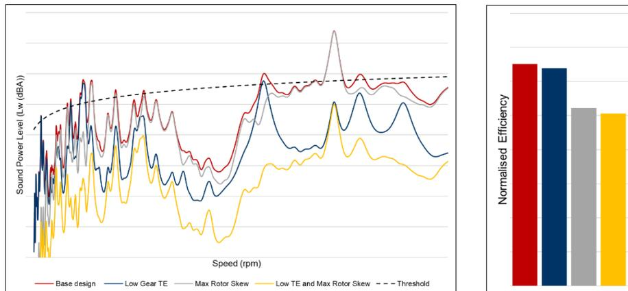
**Fig. 5.** Sound power analysis of the system when components are optimised in isolation
