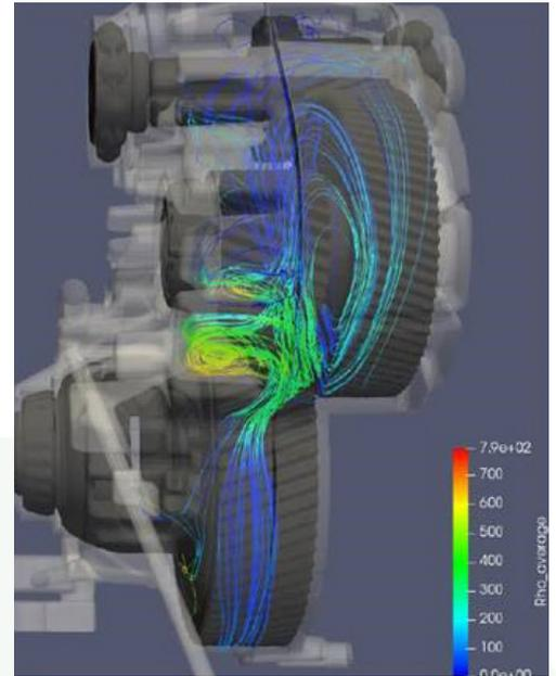
SPH model, illustrating simulated particle path
