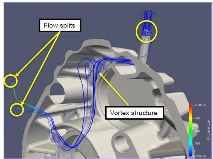
SPH model, illustrating complex phenomena in oil flow using simulated particle paths
