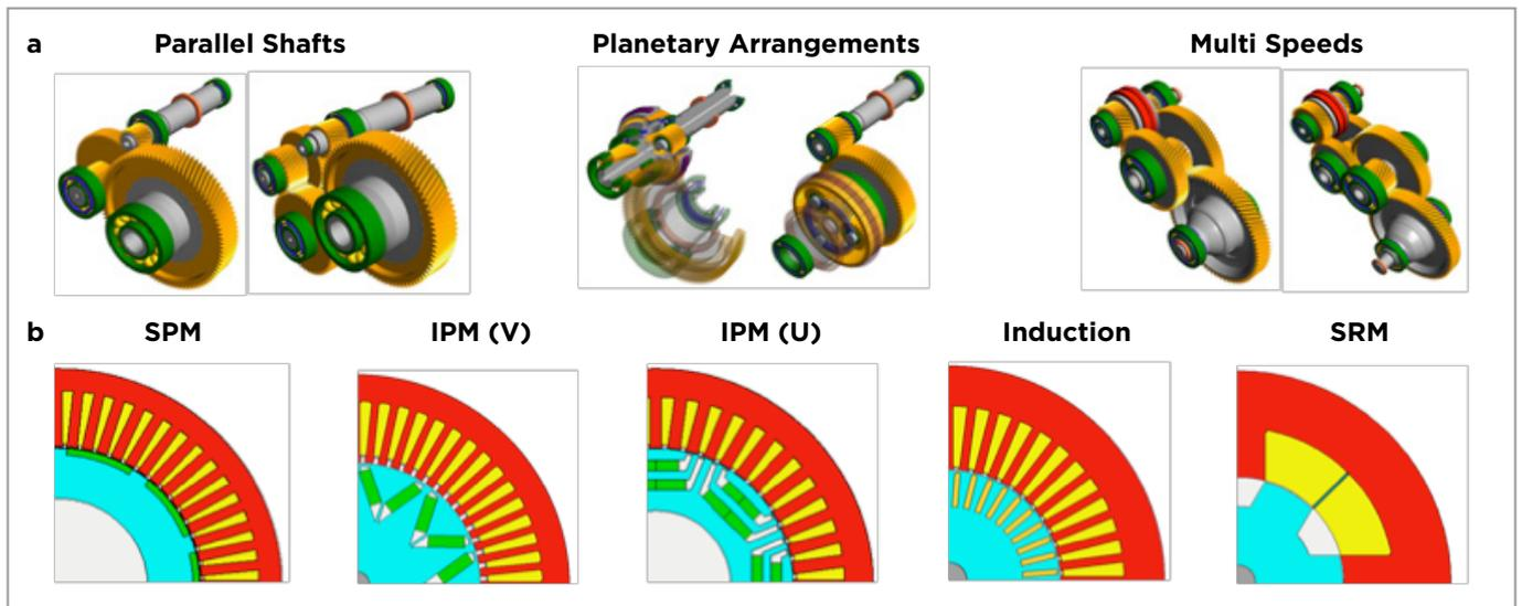
**Figure 2:** A range of transmission systems (a) and different motor types and topologies (b) can be considered using ePOP
