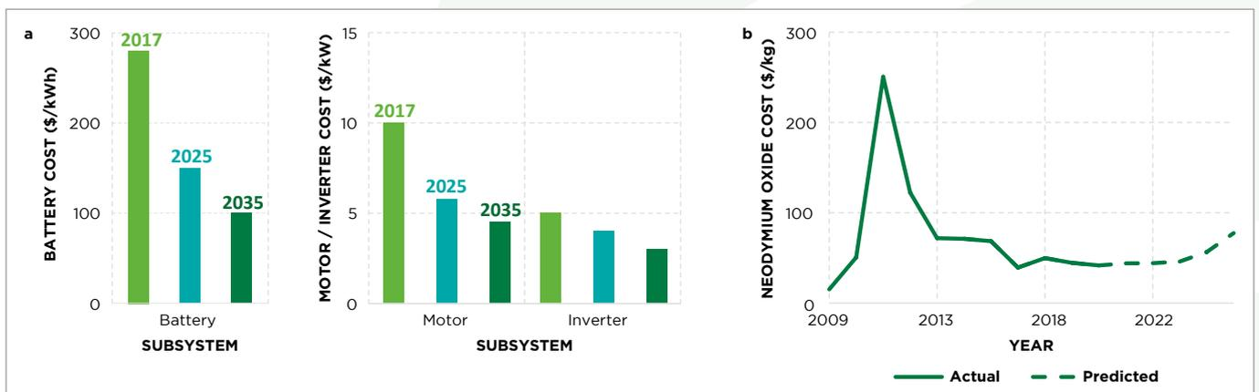
**Figure 3:** Cost trends in electrified powertrain subsystems and materials a) cost forecasts from the UK's Advanced Propulsion Centre [3], b) Neodymium oxide costs, 2009 - 2025 [4]
